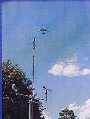
Noise monitor equipment near OIA
